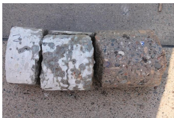
Figure 6: Mantle surface of the core 2. The carriageway slab consists of two layers. The left part is the actual structural concrete, on the right is the core of the consolidation.
